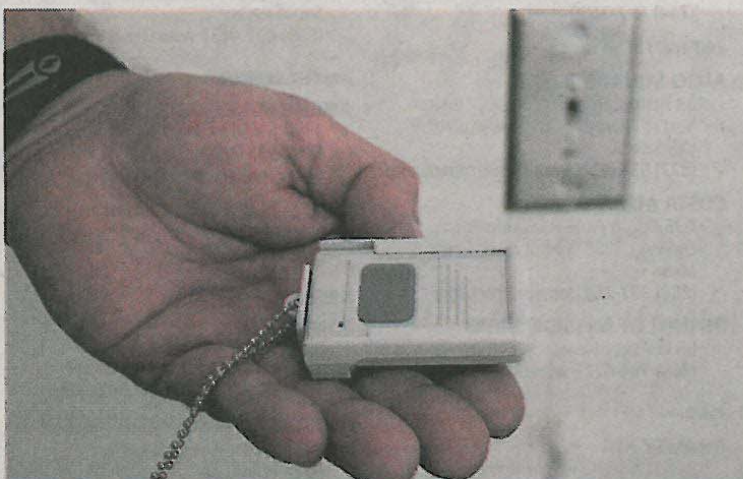
Ability First apartments come with a personal alert device and emergency pull cords that can alert staff or firefighters.
